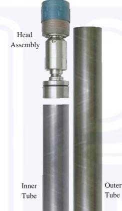
The T6 is a core barrel of sturdy design suitable for coring in all formations. The barrel is used with core bits with a relatively thin kerf to maximize the rate of penetration. T6 barrels can be used with water, mud or air flush, but when using air flush, oversize bits and core barrel couplings are commended (available on request). The barrel is available in four nominal millimeter sizes, 101, 116, 131 and 146, as well as the DCDMA hole size H.
