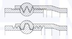
Whitworth "GAS" (DIN 2999) Socket Trapezoidal "Din" (DIN 4925) Socket
